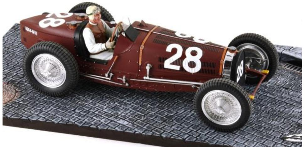
Based on the road version, the race versions have been modified significantly. In order probably to give priority to accessibility in case of repair needs, the body cut has been revised and the rear ridge has disappeared. The fuel tank caps are now screw-type and not hinged. The blades are also longer because a mesh was used to lock and unblock them.
