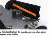
The Slot.it guide chases the mounting screws, other guides may need extra fitting.
