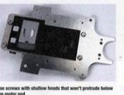
The screws with shallow heads that won't protrude below the motor pod.
