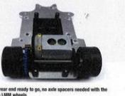
The rear end ready to go, no axle spacers needed with the wide LMM wheels.
