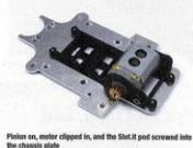
Pinion on motor clipped in, and the Slot.it pod screwed into the chassis plate.
